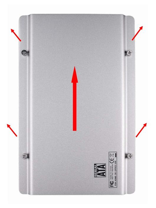
**STEP2:** Release 2 screws from back panel, and then slide out the side plates.
